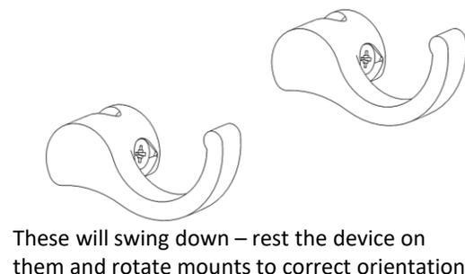
These will swing down – rest the device on them and rotate mounts to correct orientation
