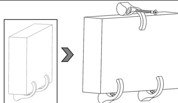
Mark the top clamp position making sure not to obstruct any of the ports you use in your setup
